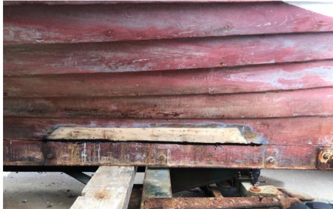
A graving piece in the garboard.
